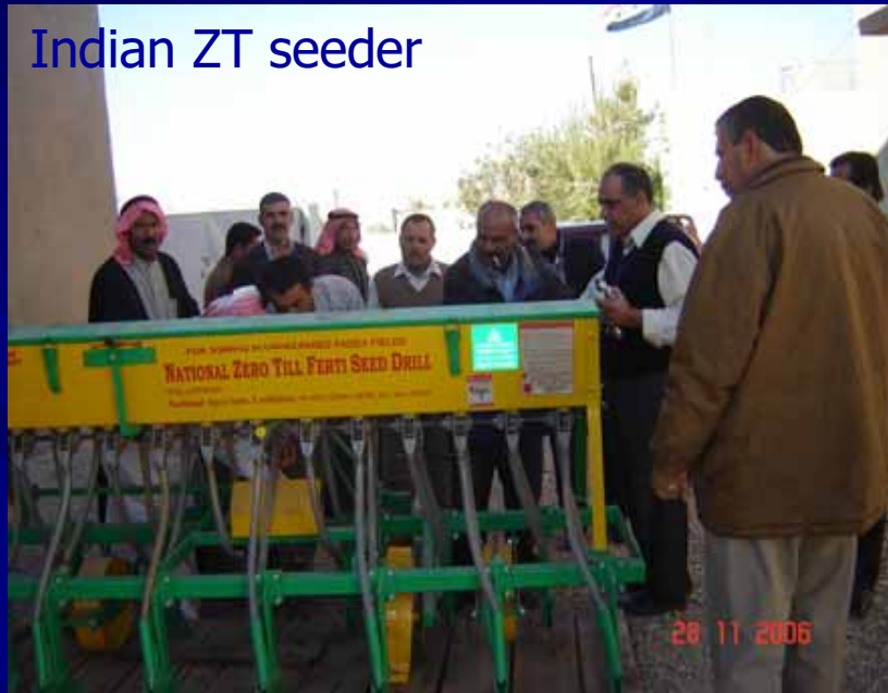
Modified Rama Seeder to ZT seeder
