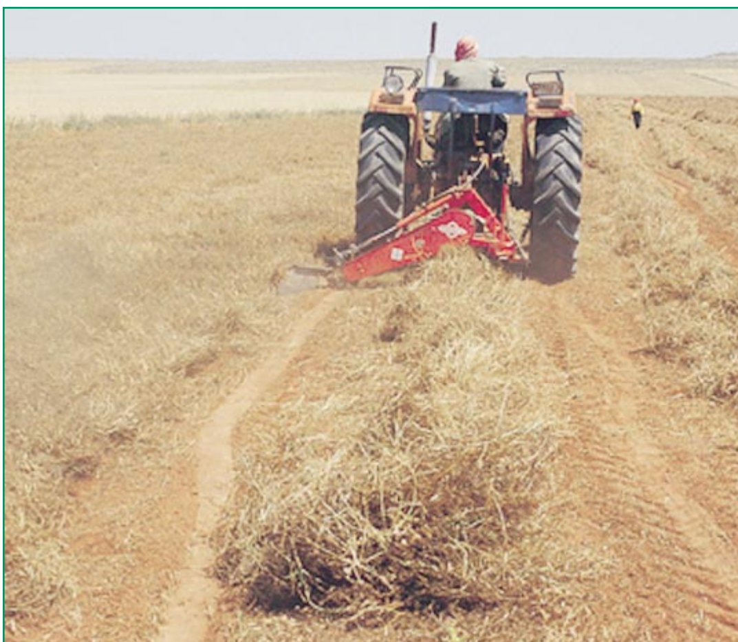
A farmer in El-Bab harvests vetch for seed, using a cutterbar mower. The availability of mowers has added to farmers' enthusiasm for growing vetch.
